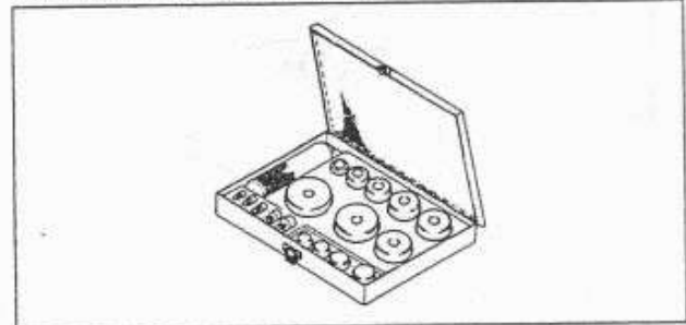
Valve Spring Compressor Adapter, \phi 22 : 57001-1202
